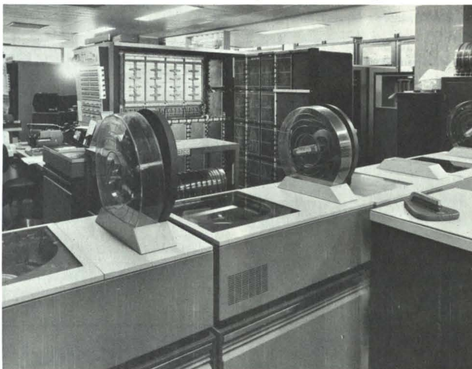
DISK STORAGE DRIVES at one of the IBM 360 Central Processing Units are part of the Postgraduate School's unique computer setup. (Official Navy photos)
