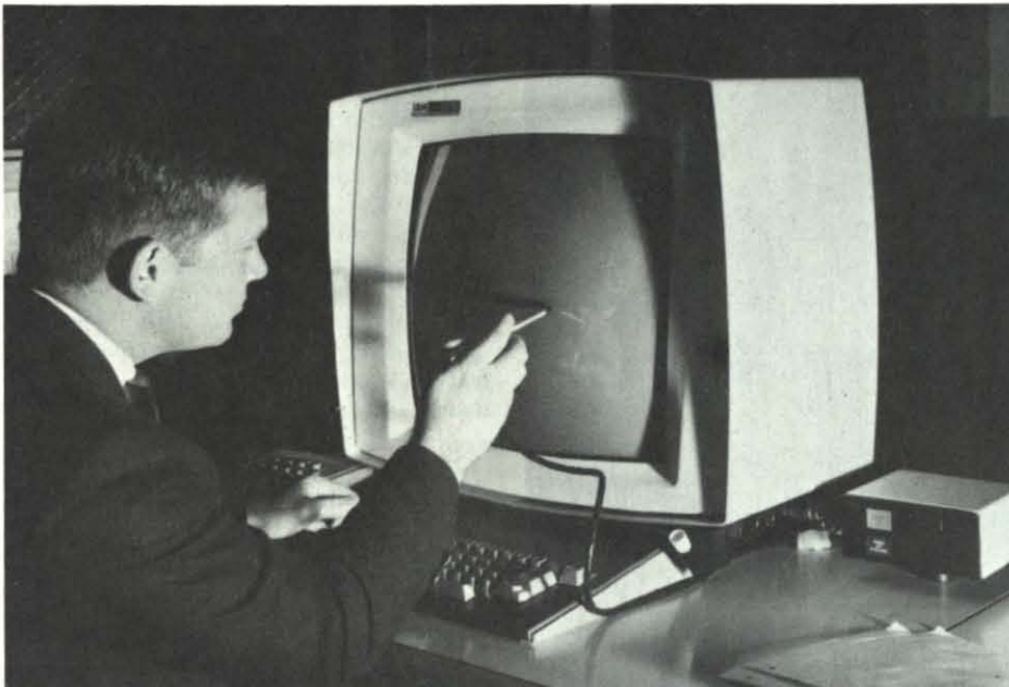
GRAPHICAL DISPLAY UNIT requires a light pen and programmed function keyboard to relay information to the computer.
