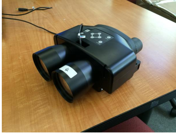
Figure 1. 3D Wireless Binocular Face Recognition System
