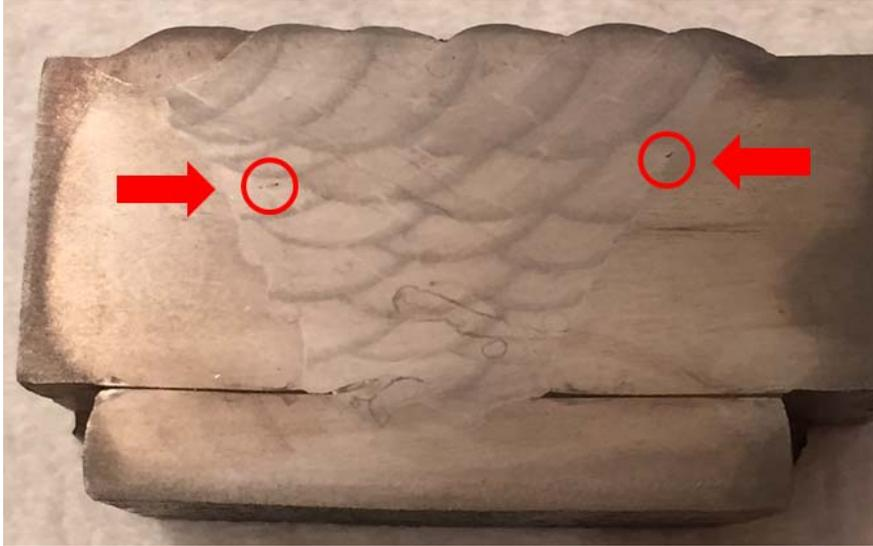
Figure 16. Porosity Found in Joint Design "A" Using 90% Ar-10%CO<sub>2</sub> Gas Mixture.
