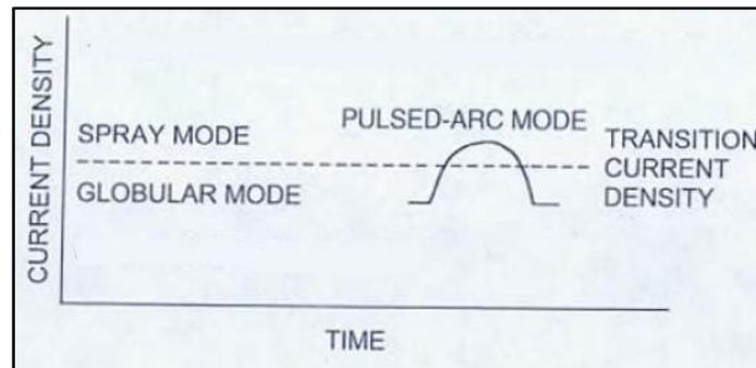
Figure 3. Gas Metal Arc Welding Transfer Mode Comparison.
