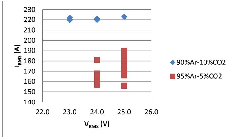
Figure 11. I<sub>RMS</sub> versus V<sub>RMS</sub> Comparison with Different Ar/CO<sub>2</sub> Gas Mixtures Using GMAW-P.
