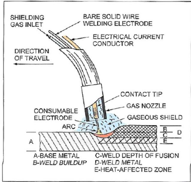
Figure 2. Schematic Representation of Gas Metal Arc Welding.
