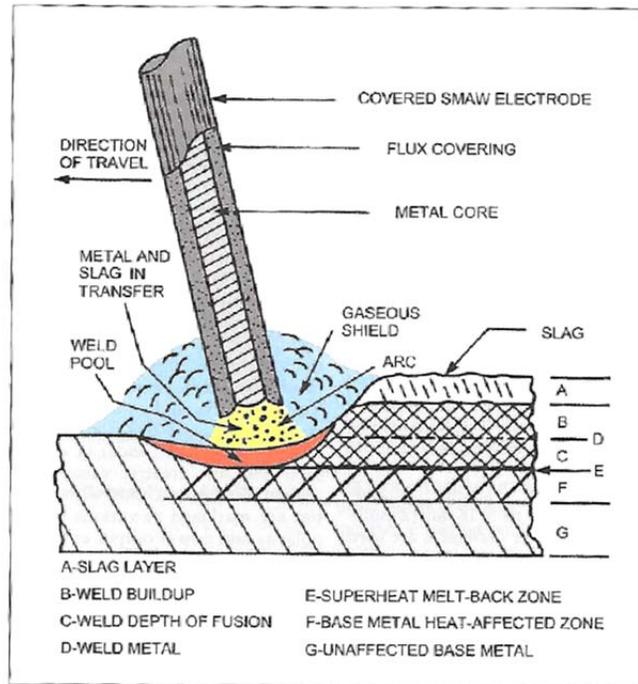
Figure 1. Schematic Representation of Shielded Metal Arc Welding.
