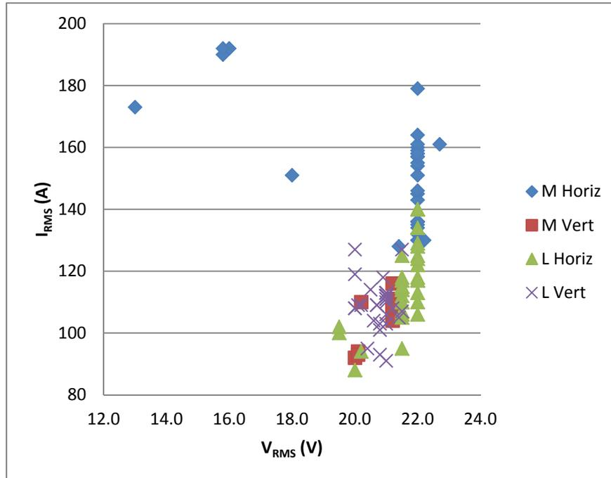
Figure 13. I<sub>RMS</sub> versus V<sub>RMS</sub> Comparison with Miller and Lincoln Welding Machines in the Horizontal and Vertical Positions Using GMAW-P.
