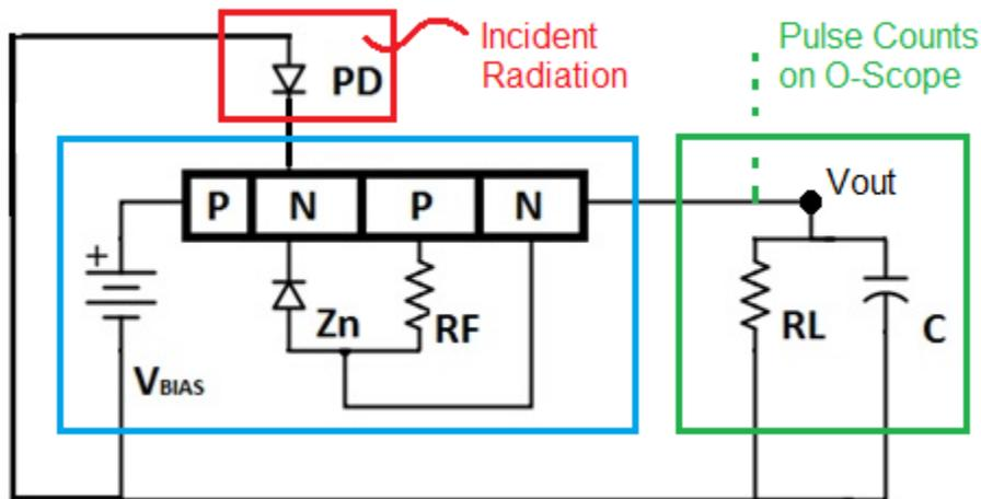
Figure 5. Basic Electrical Component Schematic of SCS Base Detector
