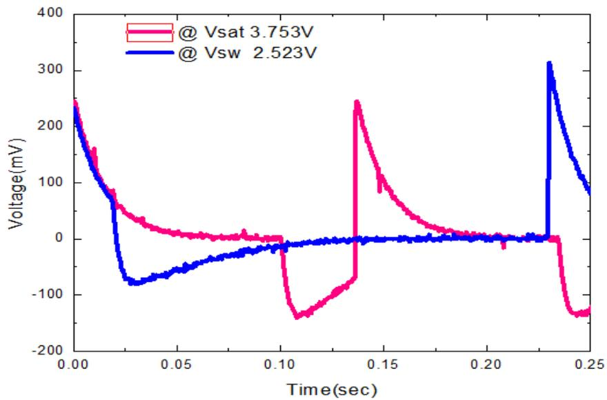
Figure 16. Pulse Saturation for  $V_{SAT}$   $R_F=5.1M\Omega$   $R_L=15.1M\Omega$
