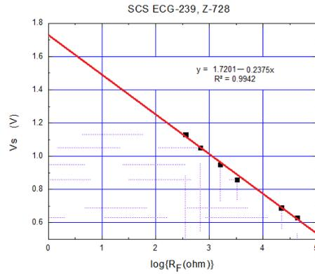
Figure 12. Switching Voltage as a Function of  $R_F$
