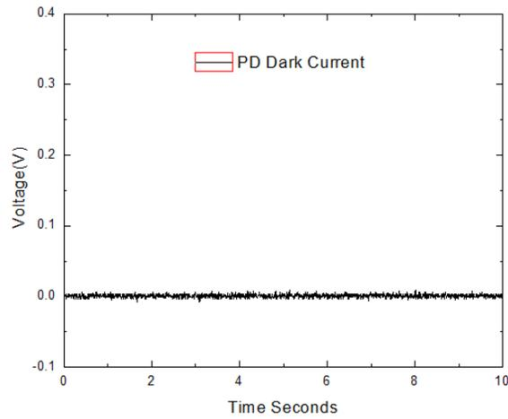
Figure 24. Response of Circuit under Dark Conditions
