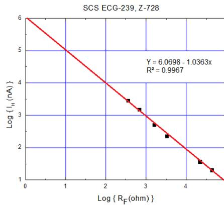
Figure 13. Holding Current as a Function of  $R_F$
