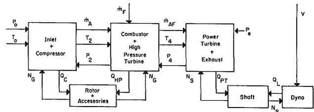
Fig. 5 Plant cause and effect model
