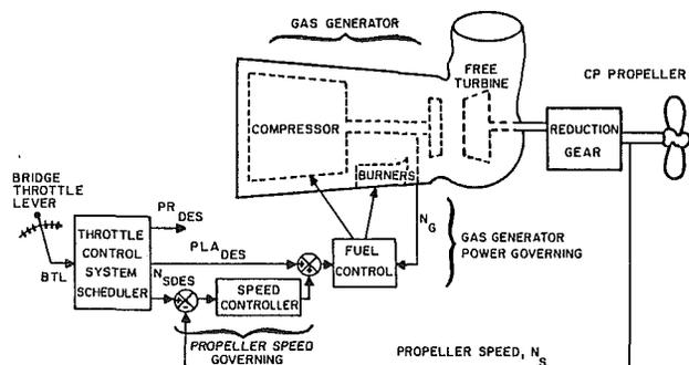
Fig. 1 Closed-loop propulsion control
