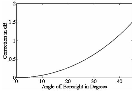
Fig. 4. Reflectivity correction to Probert-Jones equation due to off boresight electronic beam pointing.
