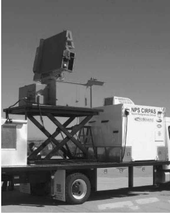
Fig. 2. Naval Postgraduate School MWR-05XP mobile, frequency agile, phased array weather radar [5].
