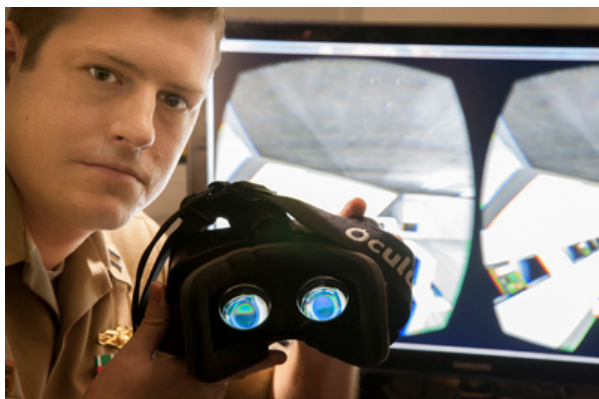
NPS computer science graduate Lt. Brendan Geoghegan demonstrates the Oculus Rift Virtual Reality (VR) head-mounted display he used as a tool to determine the viability of a novel operational view of the bridge onboard U.S. Navy warships. Geoghegan's efforts during his time as a student were awarded the top prize in the SECNAV Innovation Awards in the Innovation Scholar (Professional Military Education) Category.
