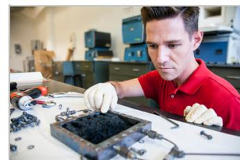
Will Curtin, a student in the mechanical engineering program, demonstrates the carbon nano-fiber foam (CFF) following its creation in the NPS Functional Materials Laboratory. For the first time, NPS researchers have developed a CFF that behaves as a viscoelastic solid with stable mechanical properties without the need of a polymeric component. Photo courtesy of NPS.
