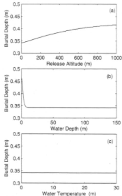
**Figure 2. Effect of varying (a) release attitude, (b) water depth, and (c) water temperature on burial depth. Values were preliminarily chosen to represent all conditions under which the IB model may be used.**
