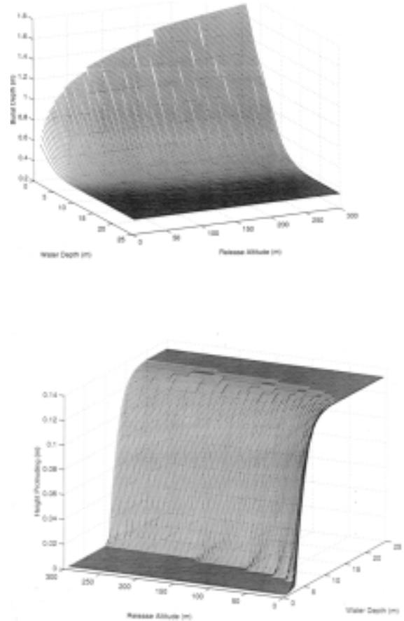
**Figure 3. Three-dimensional plot of burial depth (m) and height protruding (m) as both release altitude (m) and water depth (m) are varied. Height protruding is illustrated here to clarify the levels at which these parameters become less influential in the IB prediction.**
