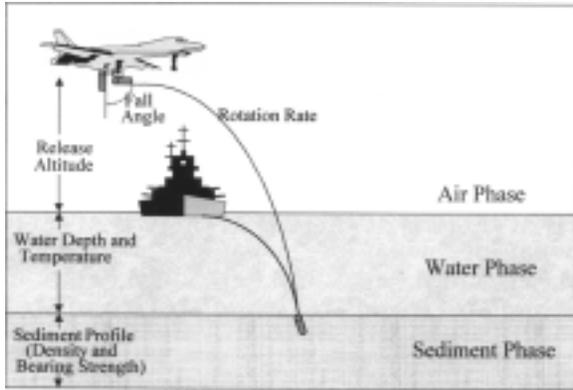
**Figure 1. The trajectory of a cylindrical mine as it falls through three phases: air, water, and sediment. Labels are parameters used by the model to calculate the velocity, attitude, and burial depth of the mine.**
