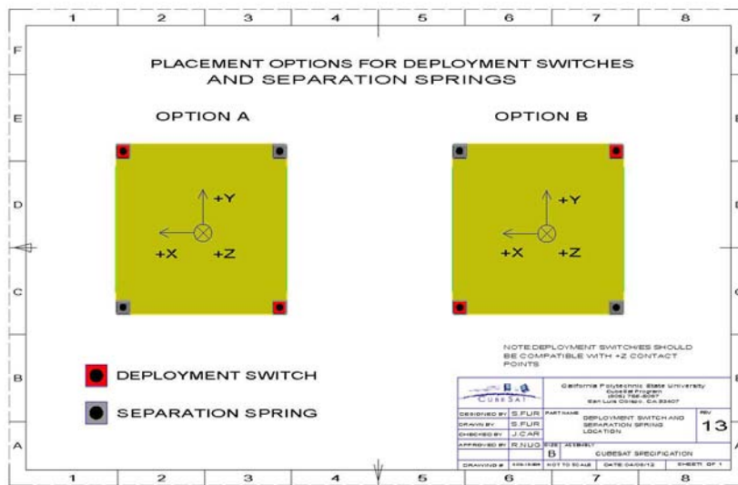
Figure 7: Deployment Switches and Separation Spring Locations
