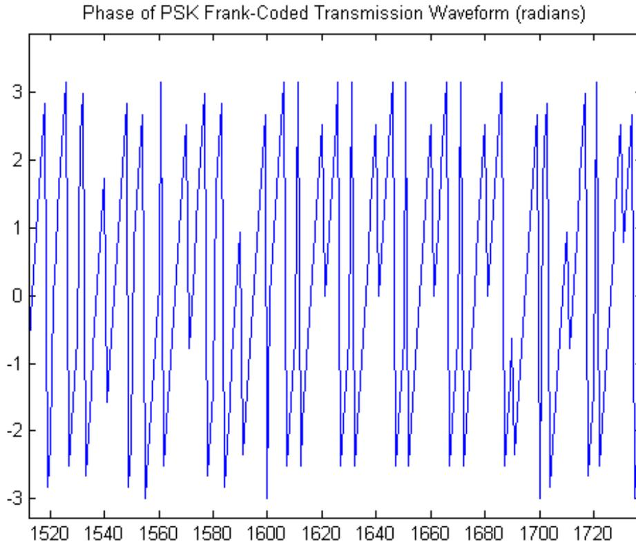
Figure 1. Phase of the Transmitted Frank-Coded Waveform
