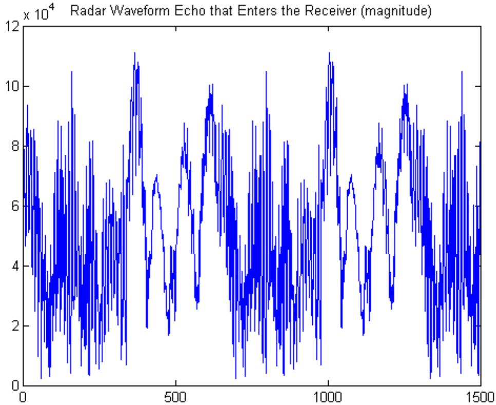
Figure 3. Radar echo due to the simulated Frank-coded waveform at the initial radar platform location along the synthetic aperture
