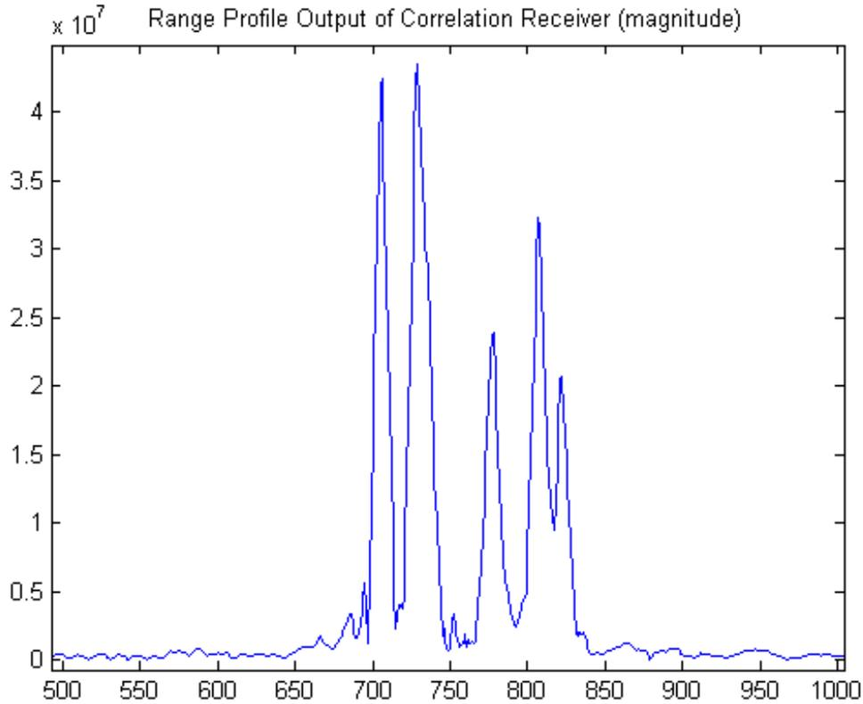
Figure 4. Output of the correlation receiver due to the simulated Frank-coded waveform at the initial radar platform location along the synthetic aperture
