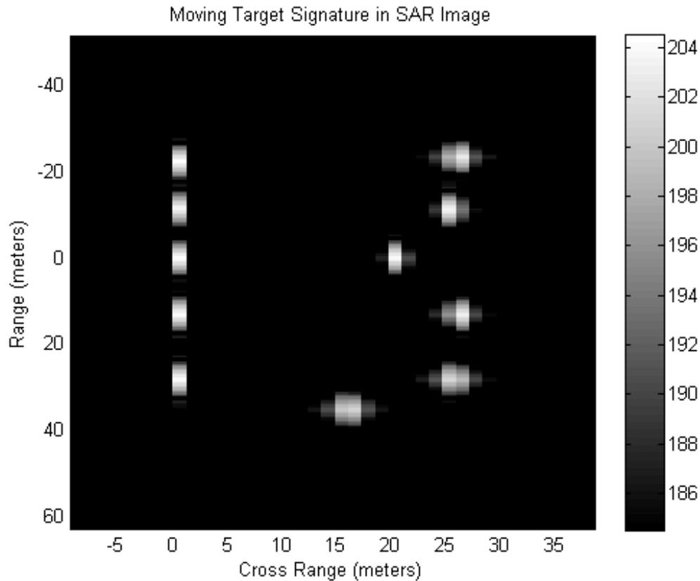
Figure 5. The resultant SAR image formed using Frank-coded transmission waveforms
