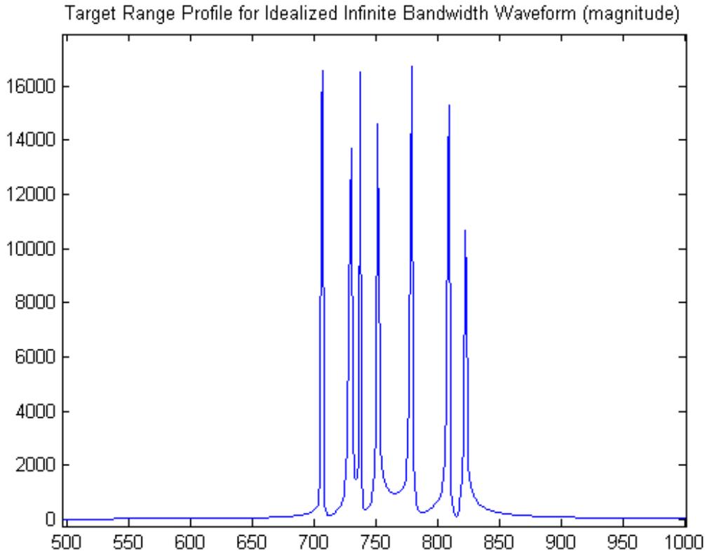
Figure 2. Idealized radar echo at the initial radar platform location along the synthetic aperture
