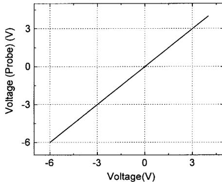
Fig. 7. Measured probe voltage versus applied input voltage.
