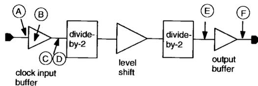
Fig. 11. Block diagram of InP divider circuit.
