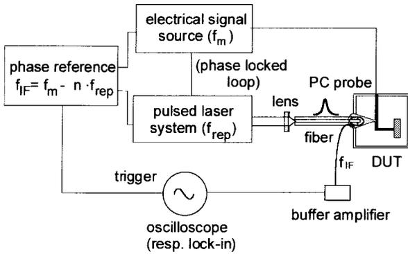
Fig. 1. Experimental setup for photoconductive in-circuit sampling measurements.
