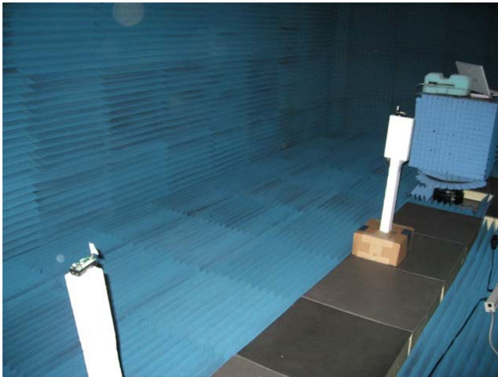
Figure 8. Anechoic Chamber used for the Experiment
