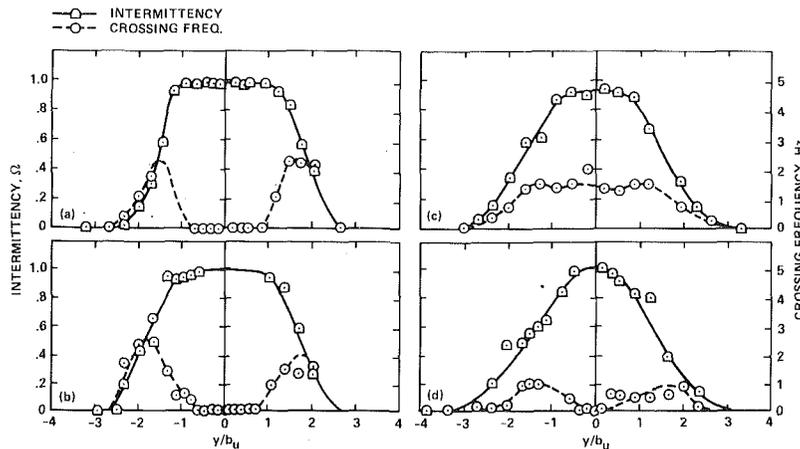
Fig. 3 Intermittency and crossing frequency distributions. (a,b) Nonbuoyant jet MSC2; (c,d) Plume MSC3. Uncertainties:  $y/b_u$ :  $\pm 0.06$ ;  $\Omega$ :  $\pm 0.05$ ; crossing frequency:  $\pm 0.25$  Hz.
