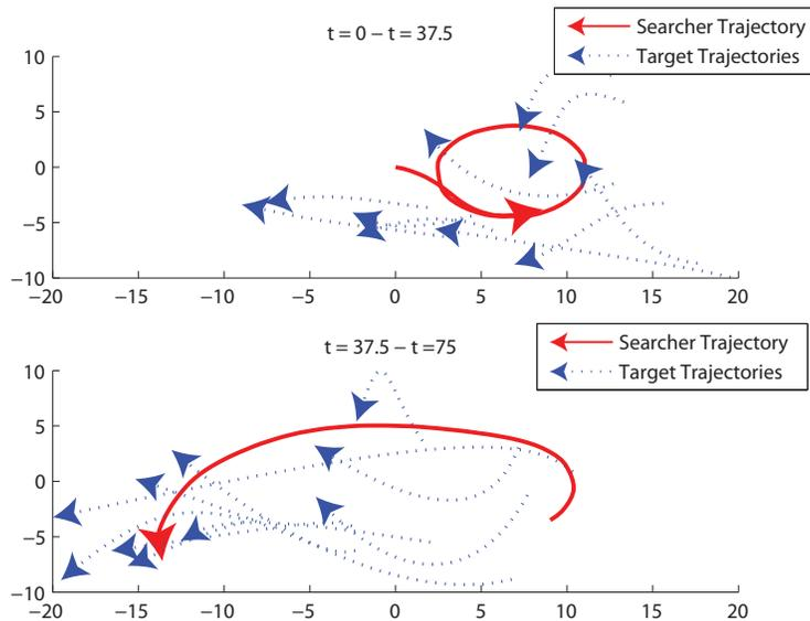
FIG. 8. Computed trajectory for a searcher attempting to detect an intruder in the channel for  $M = 5000$ . For reference, 10 possible target trajectories are shown. The target moves right to left down the channel, and the searcher starts at  $(0, 0)$  at time  $t = 0$ . The arrows in the figure indicate the orientation of the trajectories.
