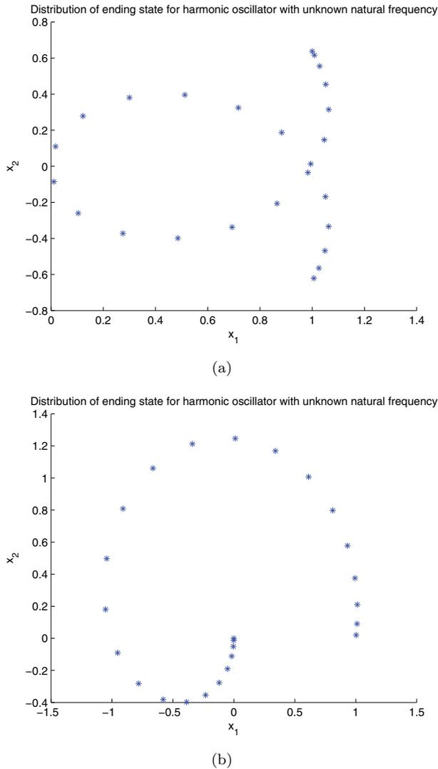
FIG. 1. Dispersion of end states of the uncertain harmonic oscillator with  $\Omega = [0, 2\pi]$  for a control designed using Pontryagin's minimum principle to stabilize (a) the median case ( $\omega = \pi$ ) and (b) the worst case ( $\omega = 2\pi$ ).
