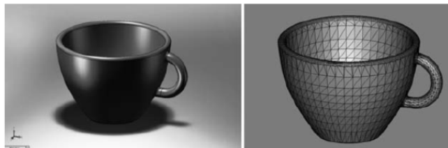
Figure 16. (Left) CAD Model, (Right) STL Format. Source: Gibson, Rosen and Stucker (2010, 23).
