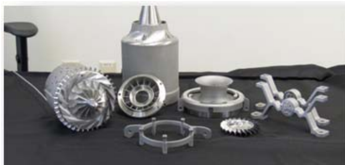
Figure 28. The Additively Manufactured Parts of the Jet Engine. Source: Szondy (2015).
