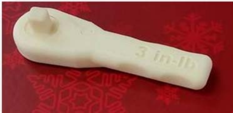
Figure 12. Ratchet Wrench Printed in the International Space Station. Source: Harbaugh (2015).
