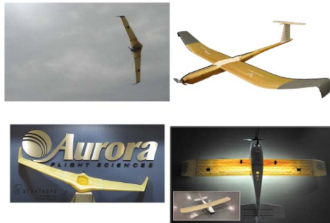
Figure 25. Examples of Small Aircraft with Additively Manufactured Parts by Aurora Flight Sciences. Source: NAS (2014, 20).
