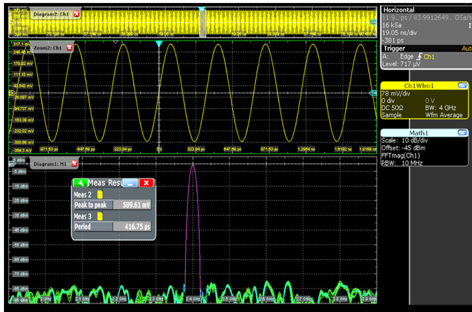
Figure 15. Screenshot of Measurement Results for RF Cable PE300-36 using R&S RTO2000 Digital Oscilloscope at 2.4 GHz with Input Power of 0 dBm
