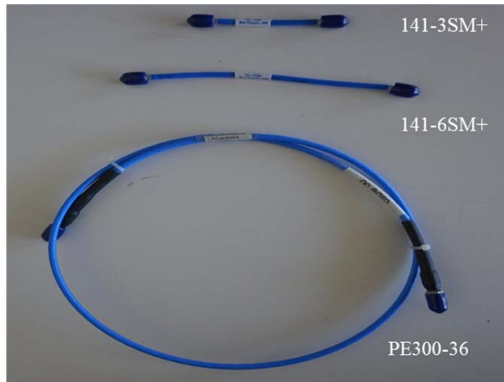
Figure 14. RF Cables PE300-36, 141-3SM+, and 141-6SM+
