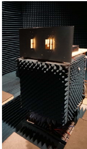
Figure 53. Placement of MWP DF System on Top of the Rotatable Pedestal
