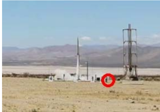
Figure 12. The Missile Trajectory-Tracking Algorithm Detecting the Smoke Plume instead of the Missile
