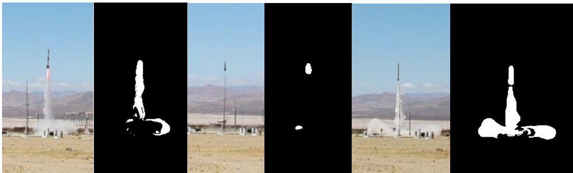
Figure 6. Missile Launches and the Corresponding Background Subtraction Frames
