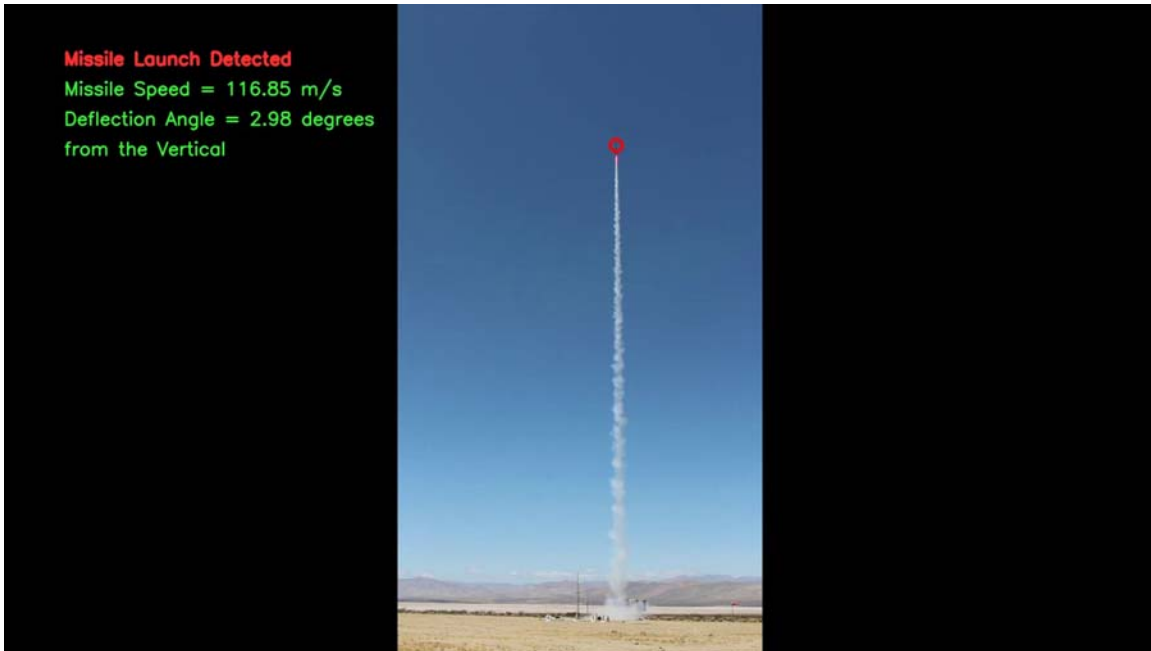
Figure 19. Rocket Speed Calculation
