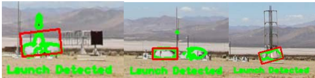
Figure 7. Missile Launch Detected by the Simulation Program
