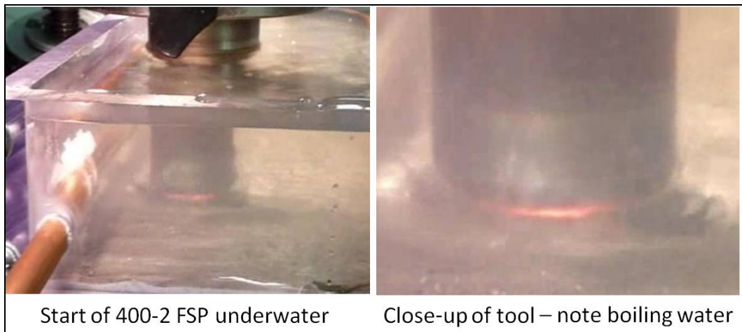
Figure 2. FSP at 400 RPM and 2 IPM (51 mm/min) while underwater.
