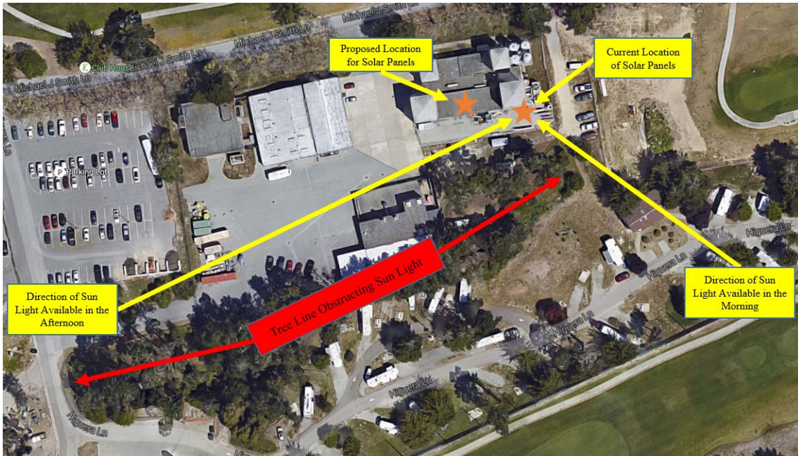
Figure 15. Solar Panels Current and Proposed Location to Improve Sun Light Availability Throughout the Day.
