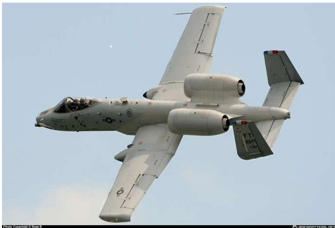
Figure 1. Fairchild A-10 Thunderbolt, a.k.a “Warthog” Note the positioning of the engine inlets relative to the inner wing section. https://img.planespotters.net/photo/302000/original/80-0194-usaf-united-states-air-force-fairchild-a-10c-thunderbolt-ii_PlanespottersNet_302341.jpg .
