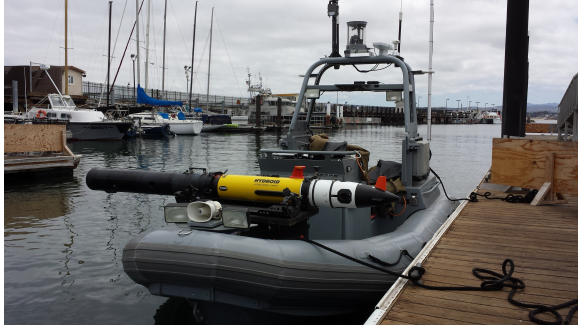
Fig. 1. The Naval Postgraduate School’s SeaFox USV and REMUS 100 AUV
