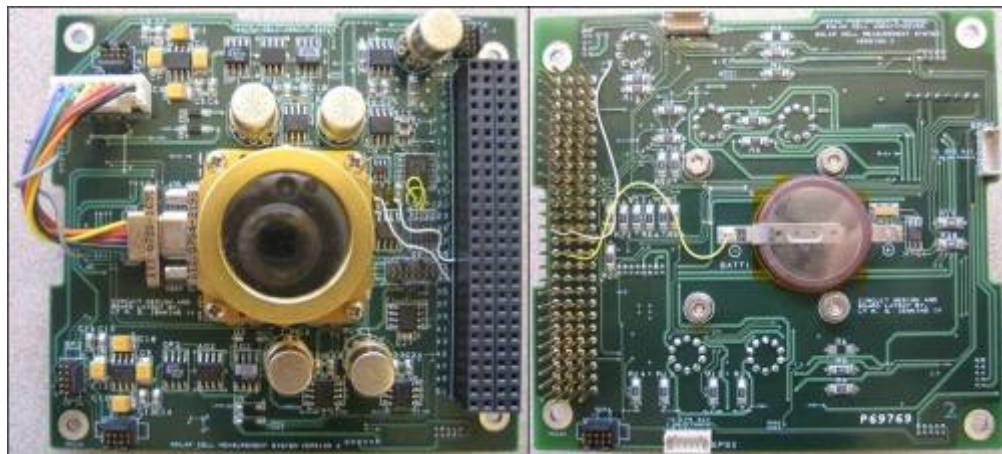
Figure 60 Completed SMS V2 PCB with Sun Sensor (front and back)
