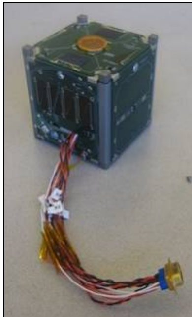
Figure 87 TVAC Test Harness Installed in NPS-SCAT
