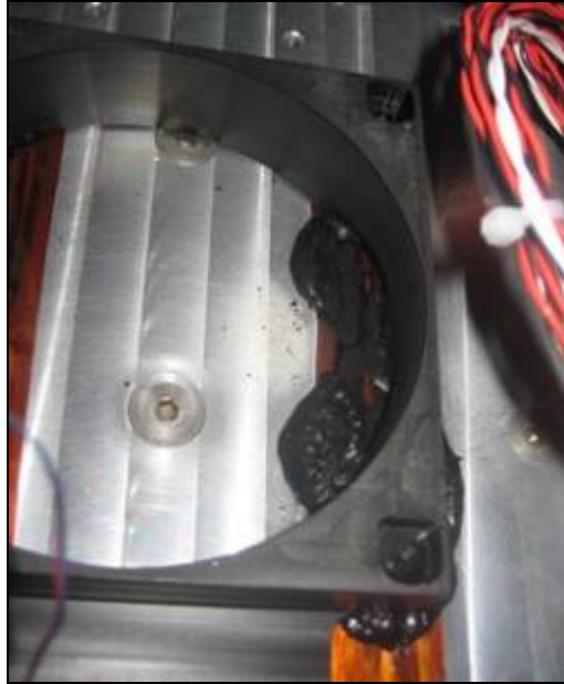
Figure 90 Melted Delrin Stand-off
