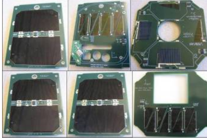
Figure 21 NPS-SCAT Solar Panels (l to r: top row: +x, +y, +z; bottom row: -x, -y, -z)
