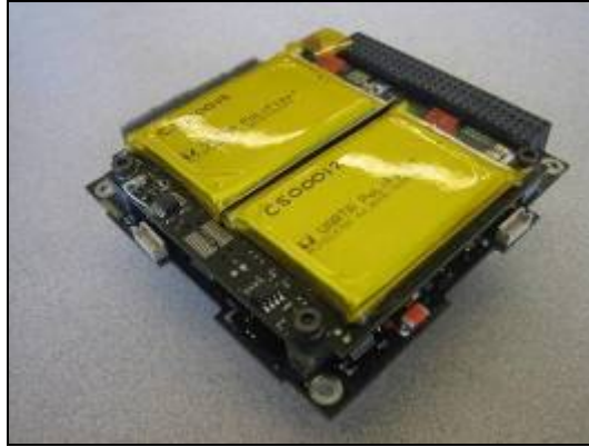
Figure 19 Clyde Space 1U EPS1 with Battery Daughter Board
