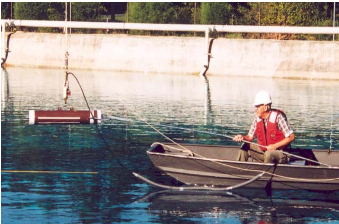
Figure 15. Blunt Nose Model Mine Shape Four Being Lowered Into Place by the Crane and Aligned for Release. Dr. Philip Valent Steadies the Mine Shape as it is Lowered into the Water.
