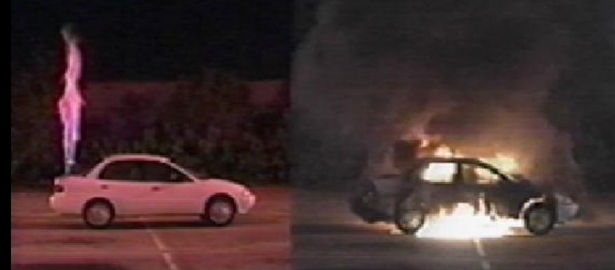
60 s: H 2 flow subsiding; max 47°C on rear window, 19.4°C on tray behind rear seat. Zooming in on gasoline car...
