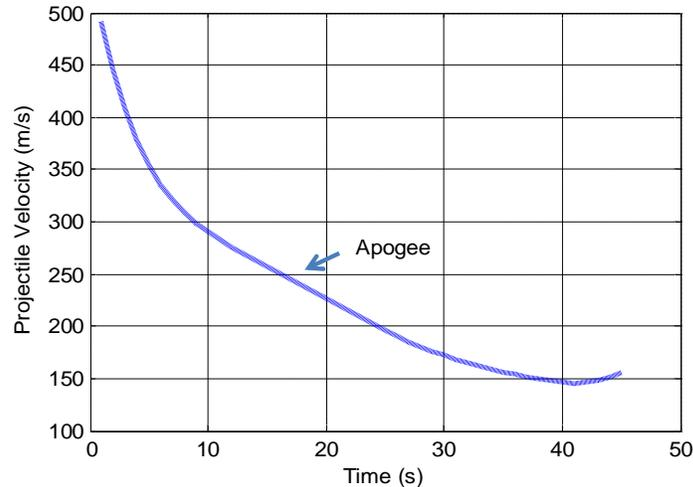
Figure 4. Typical deceleration profile of a 155 mm projectile.
