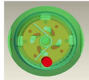
Figure 9. Mechanical release system (fuze cross section).
