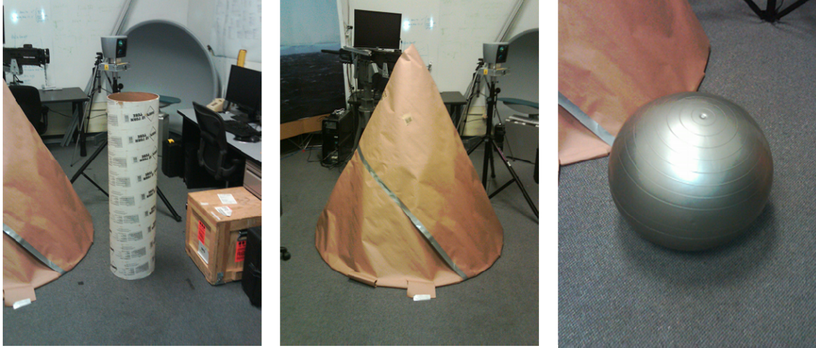
Figure 11. Photos of fiducial markers. These photos depict the three fiducial markers as used in the experimental data collection.
