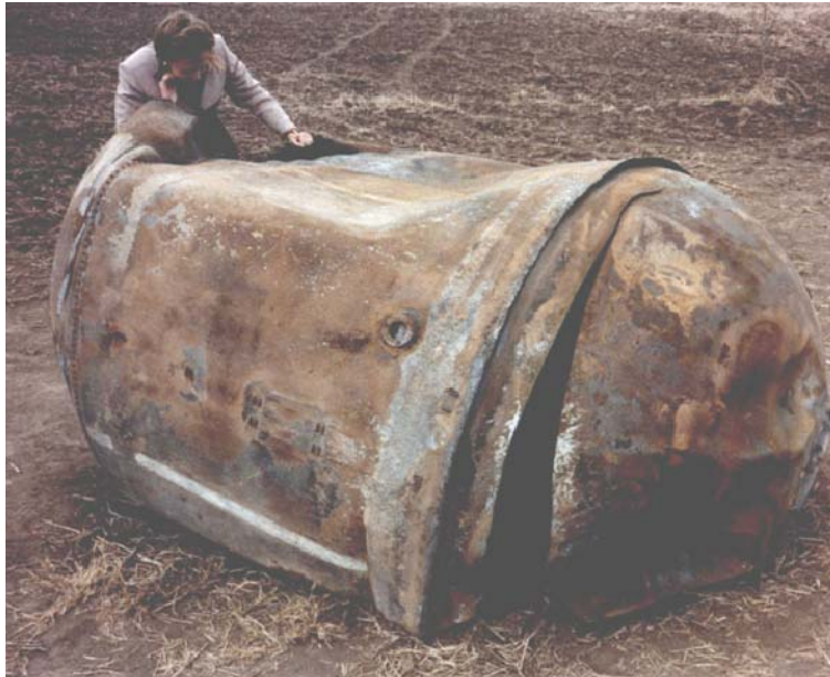
Figure 43. Delta 2 Second-Stage Main Propellant Tank After Reentry. From [48]
