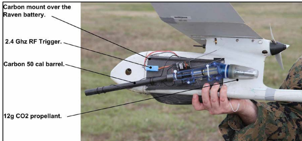
Figure 5. Small-Arms Payload Characteristics (Snyder, 2011, p. 59)
