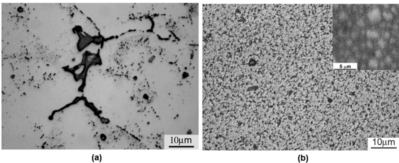
Figure 5. The as-cast AA5083 material is shown in (a) while the stir zone is illustrated in (b). Note the homogenization of microstructure in the absence of damage to the constituents or matrix.
