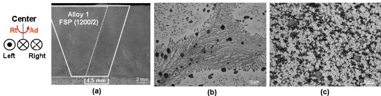
Figure 2. A montage of images of the stir zone with the pin profile superimposed is shown in (a); the base metal microstructure is shown in (b) while the refined and homogeneous stir zone microstructure is shown in (c).
