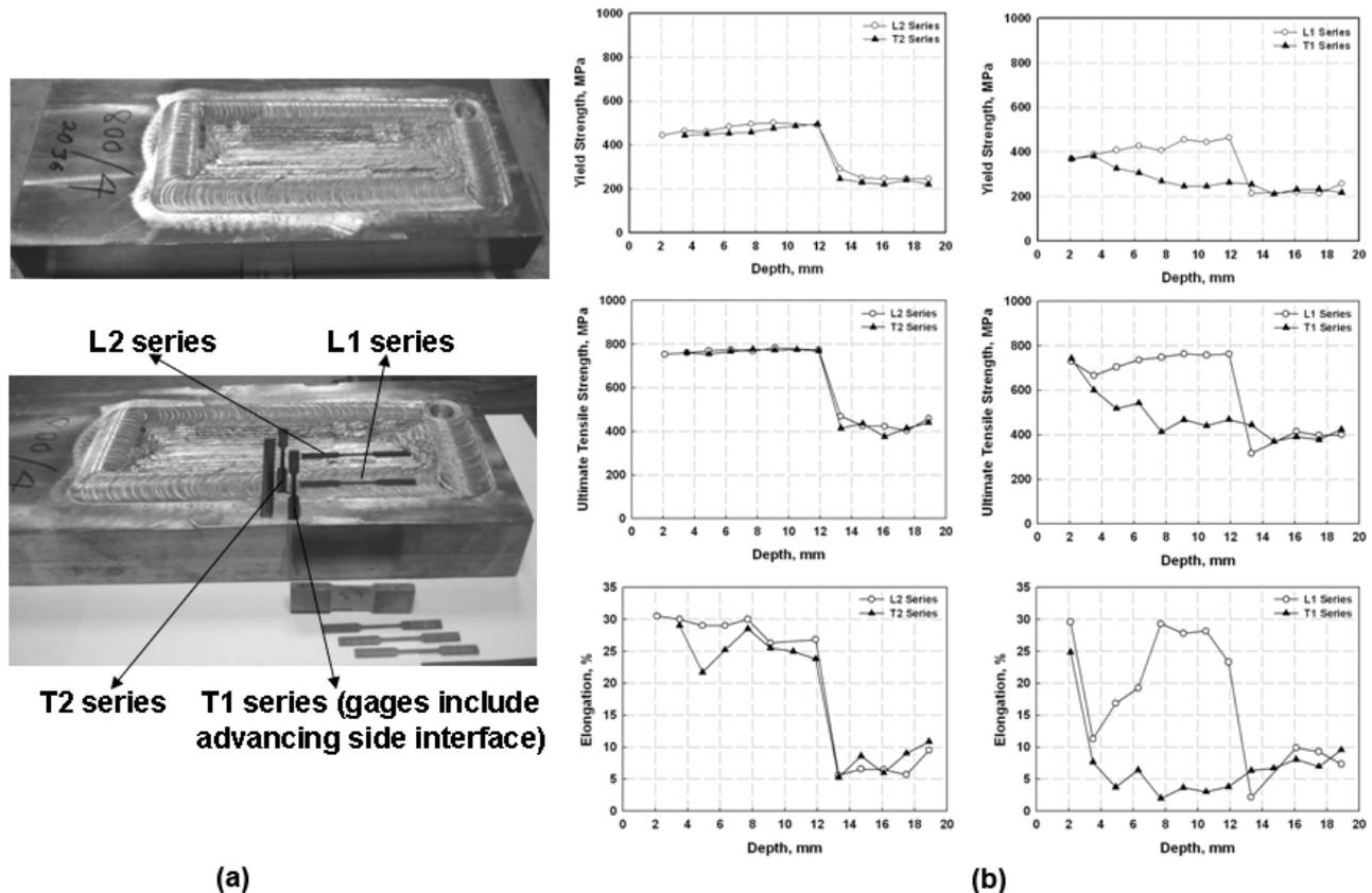
Figure 3. An as-cast plate of NiAl bronze following FSP is shown in (a); tensile test samples were sectioned by wire EDM and tensile properties were determined as a function of depth in the stir zone, as shown in (b)
