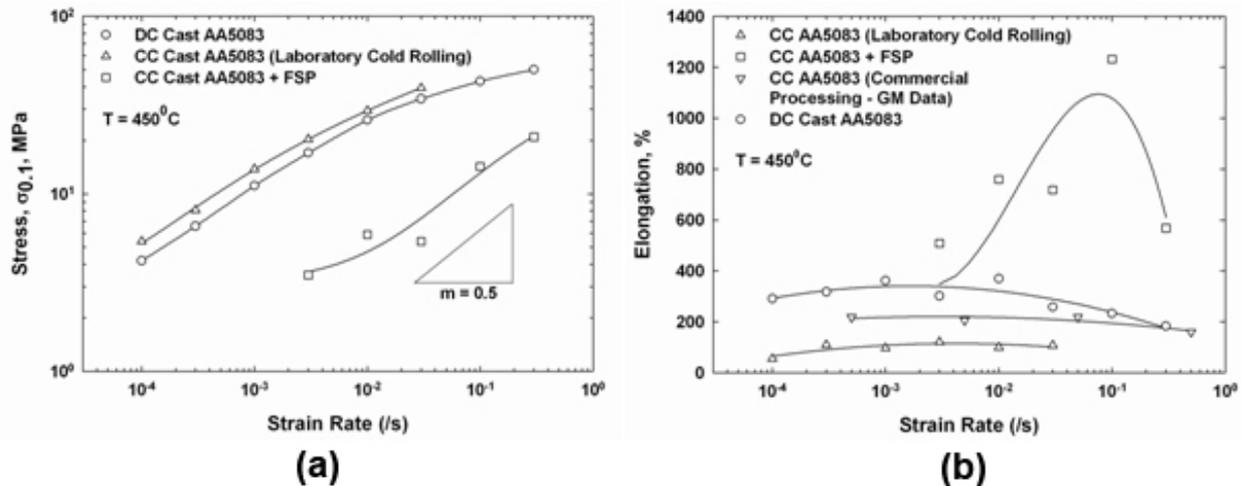
Figure 7. Plots of flow stress (at a strain of 0.1) as a function of strain rate are shown in the graph in (a) for conventionally processed AA5083 materials and the as-cast and FSP'd AA5083; the stir processed material deforms at lower stresses and higher strain rates. The peak ductility for the stir processed material corresponds to the peak  $m$ -value of 0.5. The high ductility after processing likely also reflects reduced cavitation.
