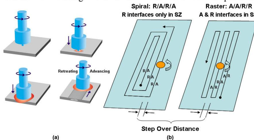
Figure 1. A schematic of FSP [1] is shown in (a); spiral and raster patterns for FSP are illustrated in the schematics in (b), which show that spiral patterns may leave only retreating interfaces (except on the first pass) while raster patterns leave both advancing and retreating interfaces in the SZ.
