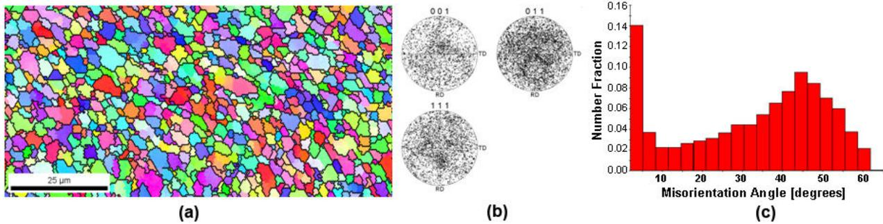
Figure 6. An OIM grain map in (a) demonstrates refinement of the stir zone to grains  $\sim 1.2\mu\text{m}$  in size; a near random texture and misorientation distribution in (b) and (c), respectively, are consistent with recrystallization while a low-angle peak in the misorientation distribution is consistent with residual deformation due to the tool shoulder.
