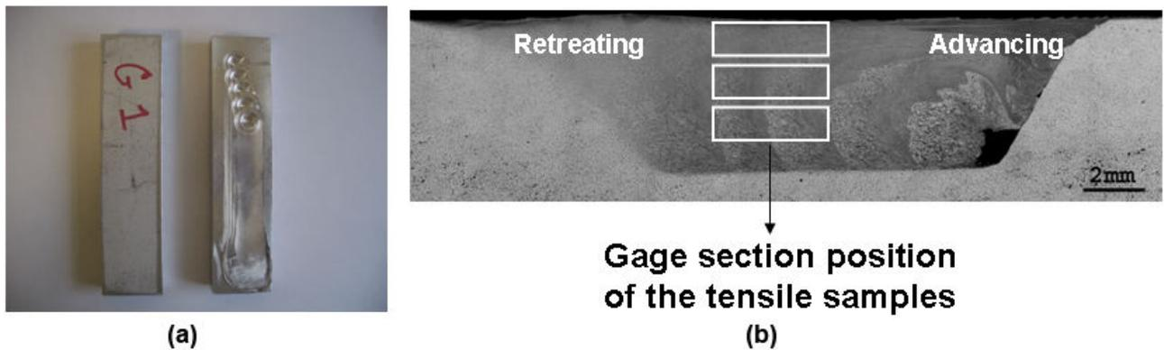
Figure 4. Five FSP traverses were conducted on as-cast AA5083 material as shown in (a); a transverse view of the resulting stir zone is depicted in (b). A tunnel defect is apparent at lower right.
