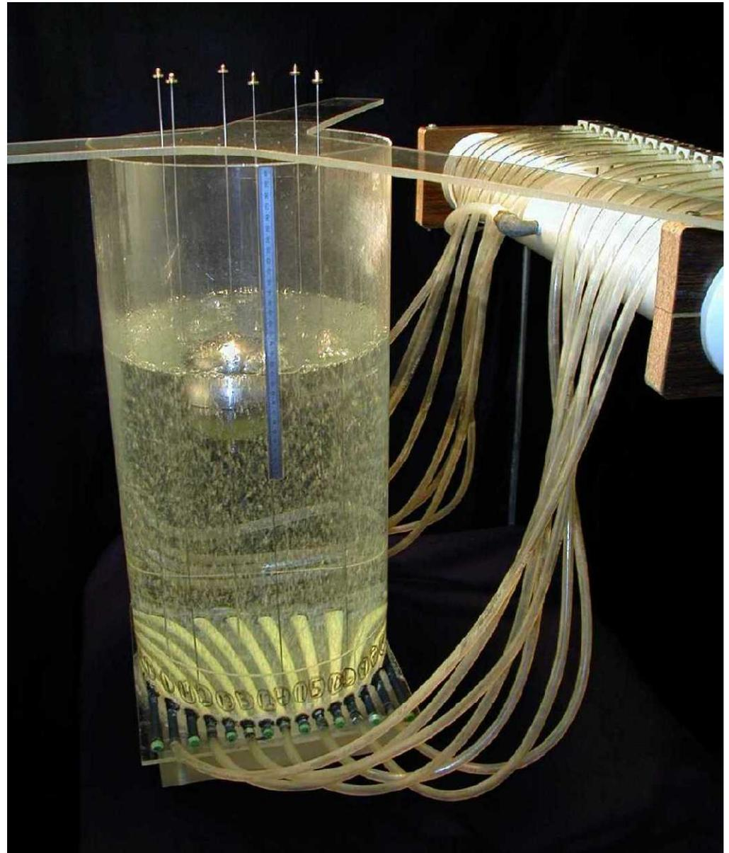
Critical to experiment is “balancing” bubble flow, so that uniform bubble field occurs. Otherwise, localized flow regions occur. Result:
