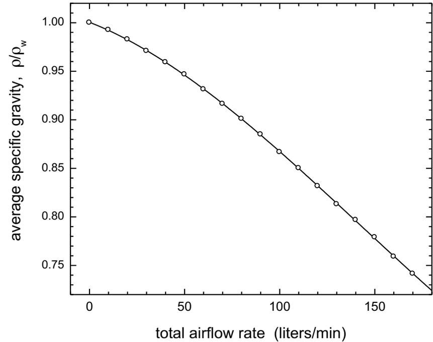
Height of fluid column varies nonlinearly with airflow rate, because bubbles remain in tank for longer time due to height increase.
