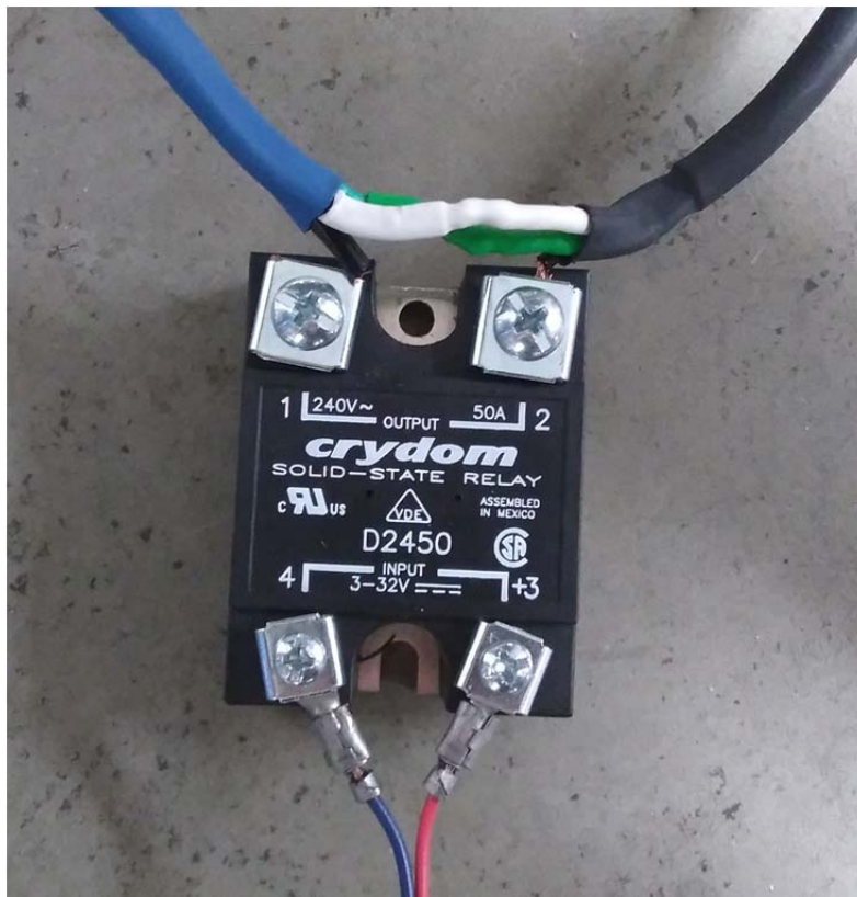
Figure 40 SSR with Solenoid and Micro 850 Attached
