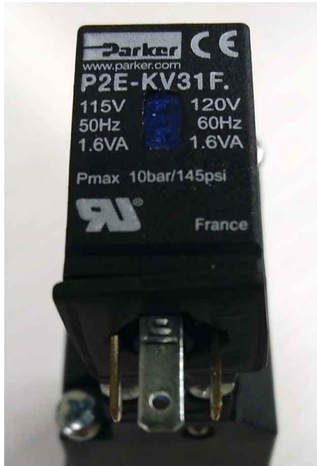
Figure 42 Solenoid Male Connection
