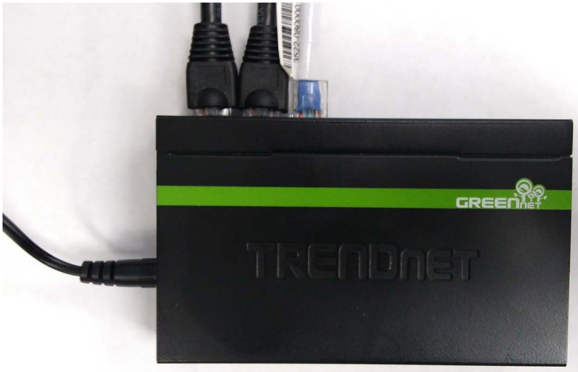
Figure 34 Ethernet Switch Used to Interface Controller and HMI
