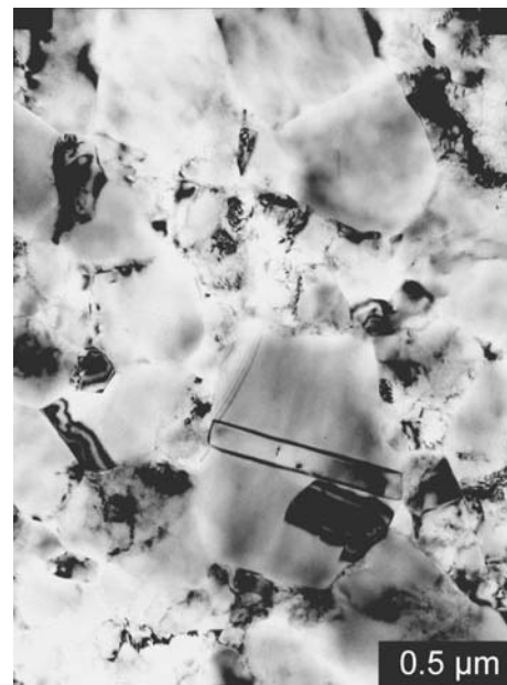
Fig. 2 TEM microstructure of HPT copper [16]
