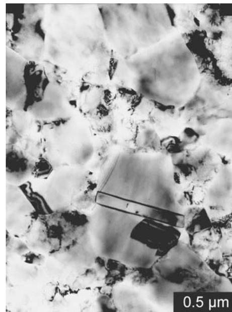
**Fig. 2** TEM microstructure of HPT copper [16]
