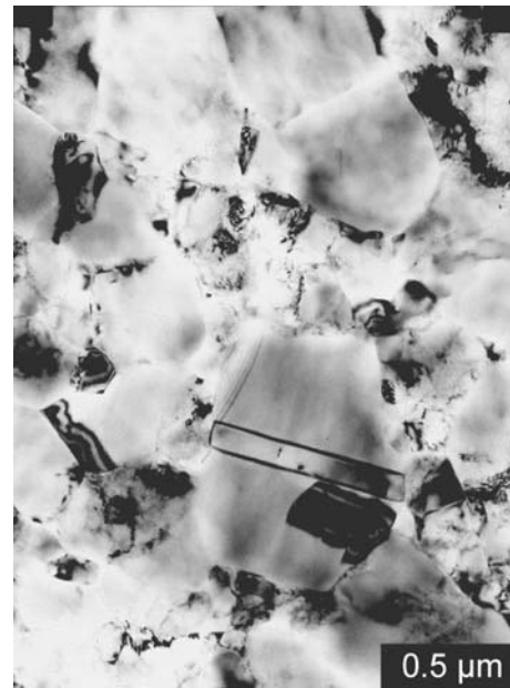
Fig. 2 TEM microstructure of HPT copper [16]
