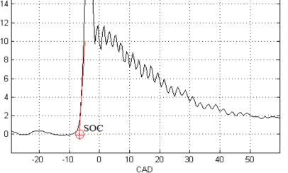
Cetane number relates to the ignition delay of diesel fuel. This ignition delay is determined by the time it takes between fuel injection into the cylinder and the first identifiable pressure increase due to combustion. Increasing the cetane number can reduce pollutant emissions, avoid difficulties in an engine during cold-starting, and increased combustions characteristics .
