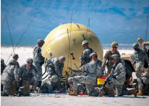
The Army will use two sizes of the inflatable satellite antenna for the Low Rate Initial Production of Transportable Tactical Command Communications (T2C2) Lite (v1) and T2C2 Heavy (v2). During Joint Forcible Entry operations at Network Integration Evaluation 16.1 in October 2015, the 82nd Airborne Division successfully utilized the capability to provide early entry network communications during the mission. (Photo by Jett Loe, Sun-News)
