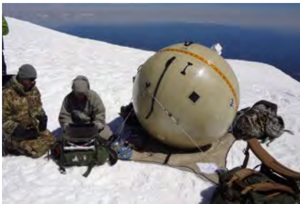
Because the T2C2 solution is inflatable, it can provide a larger dish size with increased capability and bandwidth efficiency in a smaller package. The Army will use two sizes of the inflatable satellite antenna for the Low Rate Initial Production of Transportable Tactical Command Communications (T2C2) Lite (v1) and T2C2 Heavy (v2). (U.S. Army photo)
