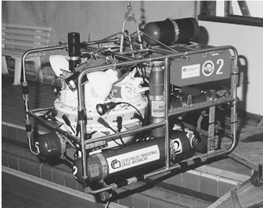
Fig. 7. Roby2: the digital gyro compass cylinder is visible on the top rear of the vehicle, while the profiling sonar is positioned on the top front of the vehicle.
