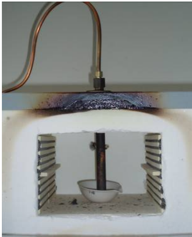
Figure 3. Photograph showing the copper test tube connected to the vacuum/argon tubing inside the furnace.
