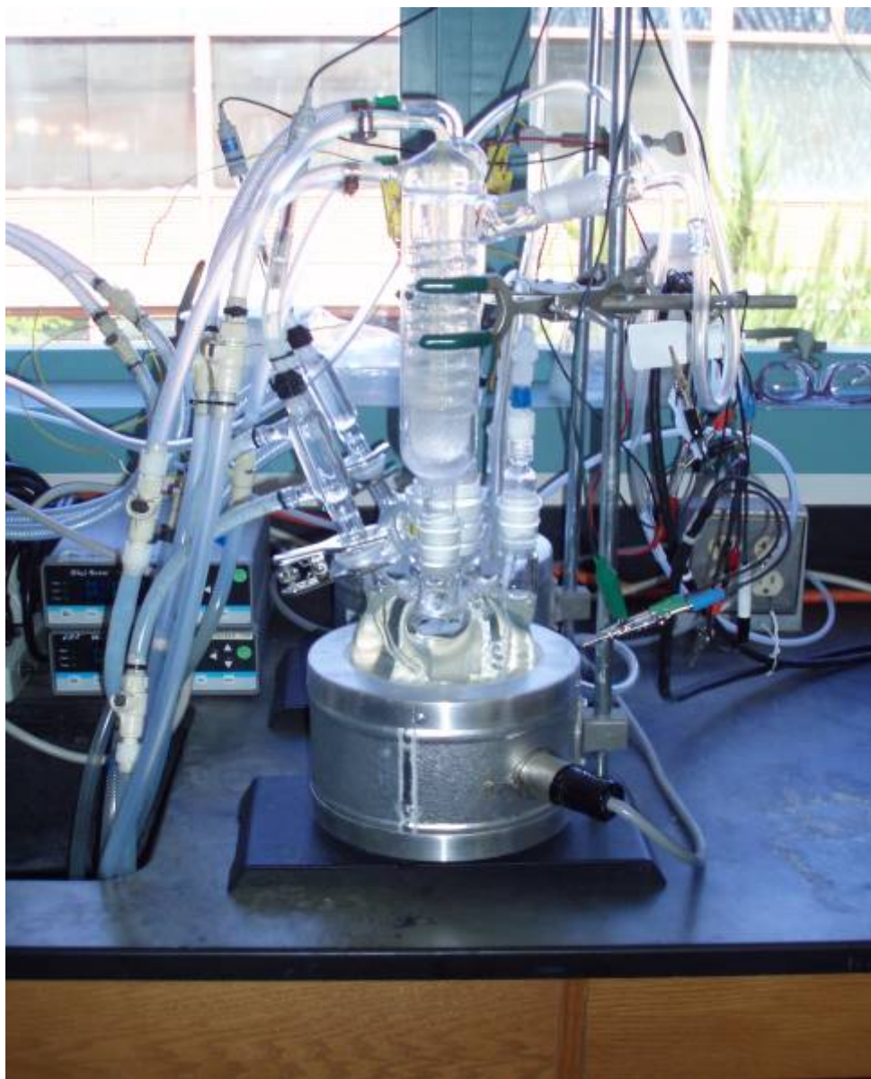
Figure 7. Photograph of the cyclic polarization test apparatus.
