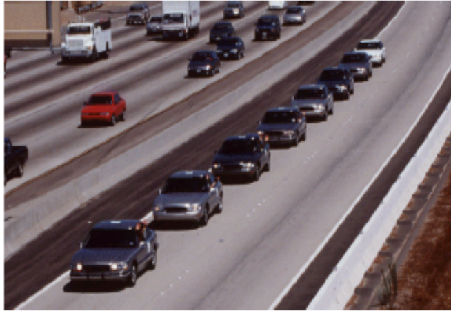
Figure 1. Platoon of automated vehicles on an Automated Highway System, developed by the PATH project (From: [2])
