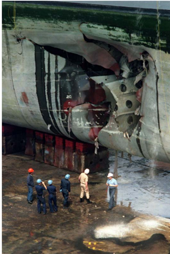
Figure 5. Damage to the USS Tripoli after Striking a Contact Mine during Desert Storm. Source: Gawlowicz (1991).
