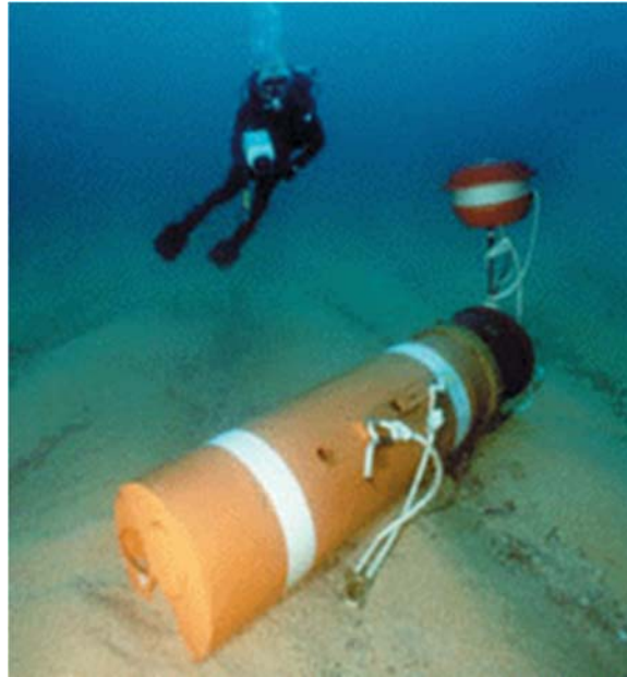
Figure 6. Influence Type Bottom Mine. Source: U.S. Navy (2002).
