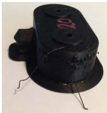
Figure 22. Part with Material Splatter
