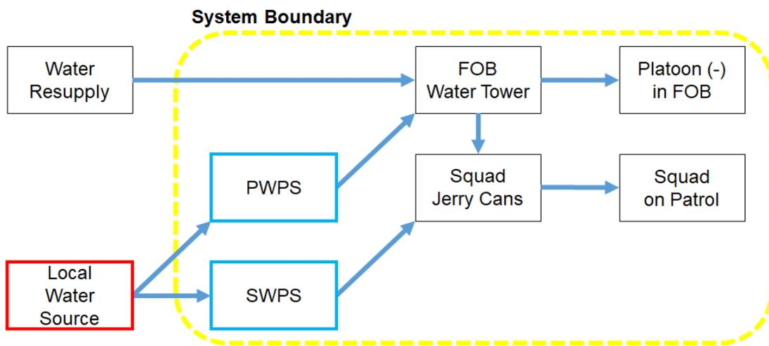
Figure 5. Simulation Model of Foraging System. Source: Soh (2017).
