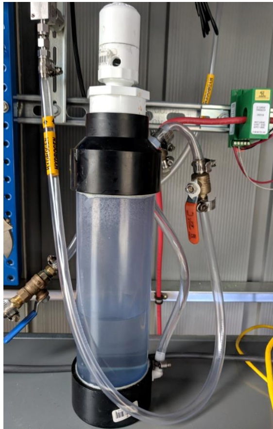
Figure 9. Hydrogen Bubbler with Pressure Relief Valve
