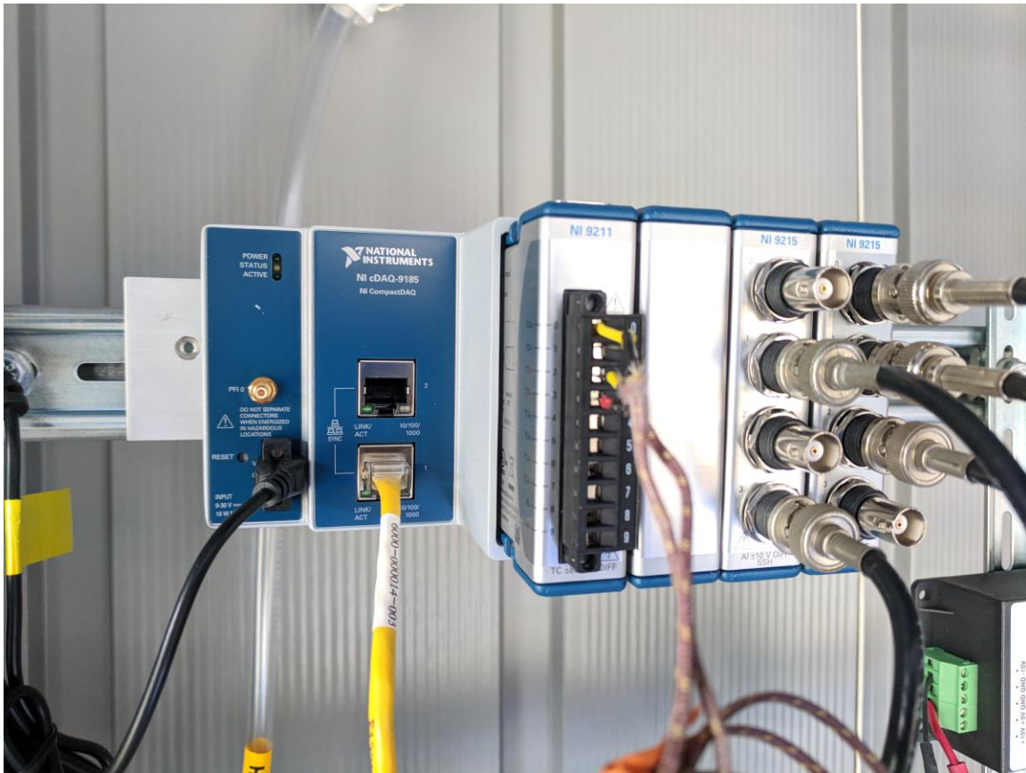
Figure 26. National Instruments CompactDAQ Model cDAQ-9184 with Analog Thermocouple and Voltage Input modules.
