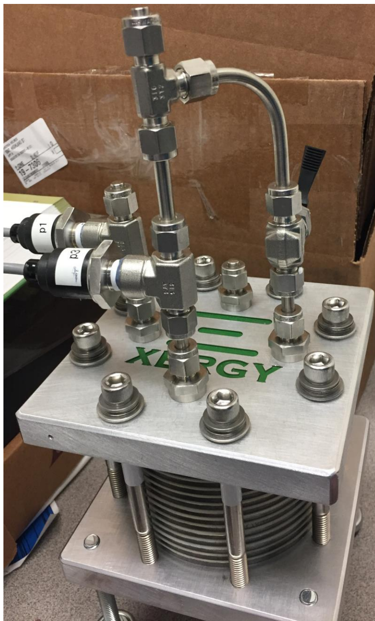
Figure 17. 0.4 slpm Electrochemical Hydrogen Compressor with 15 Proton Exchange Membranes
