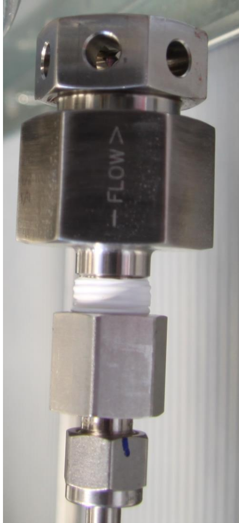
Figure 12. Screw-Type Rupture Disc Assembly with Muffled Outlet Port
