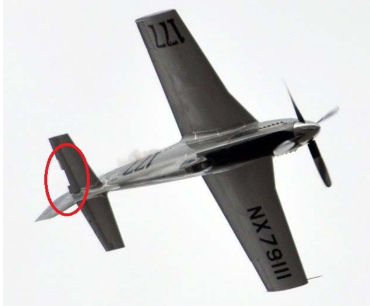
Figure 9. Trim Tab Missing on Aircraft 248
