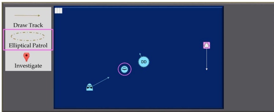
Figure 68. Notional workflow where the user selects the UAV to task (pink circle left of center) and then selects pre-defined tasking from left navigation bar (grey box at top left).
