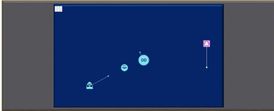
Figure 67. Notional interface for tasking single drone showing common operational picture with the drone (DD at center), a commercial vessel (pink at right), and a UAV and USV (blue at bottom left).
