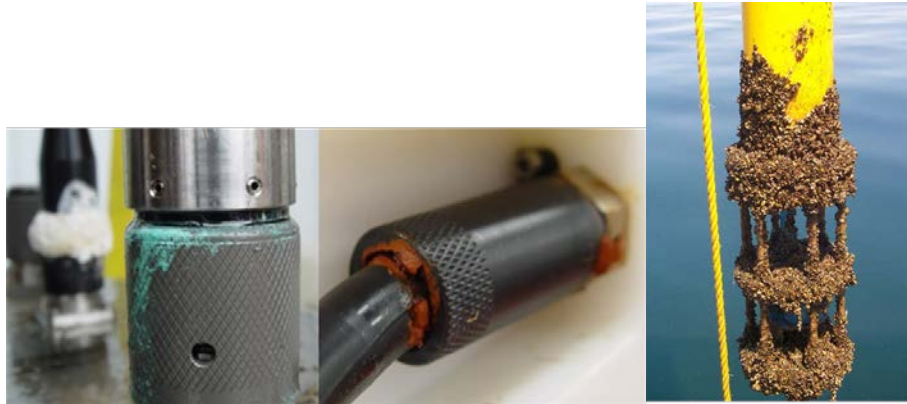
Figure 12. Corrosion 5 (left) and biofouling 6 (right) are common causes of sensor failure.
