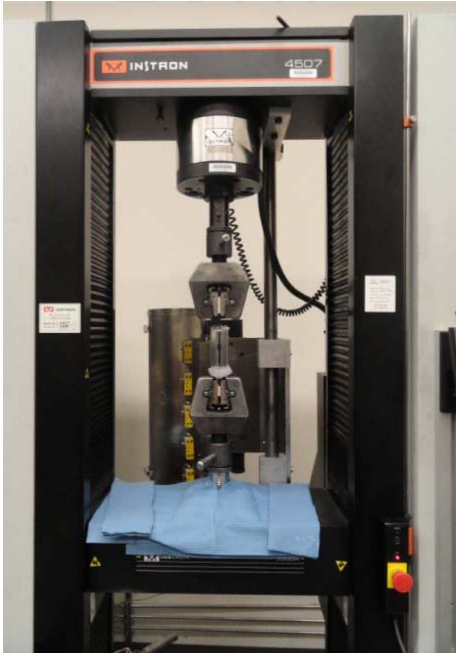
Figure 17. Instron 4507 test frame used in the SSRT testing of laser peened samples.
