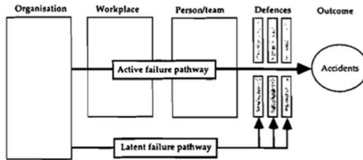
Figure 3. Active and Latent Failure Pathways 136
