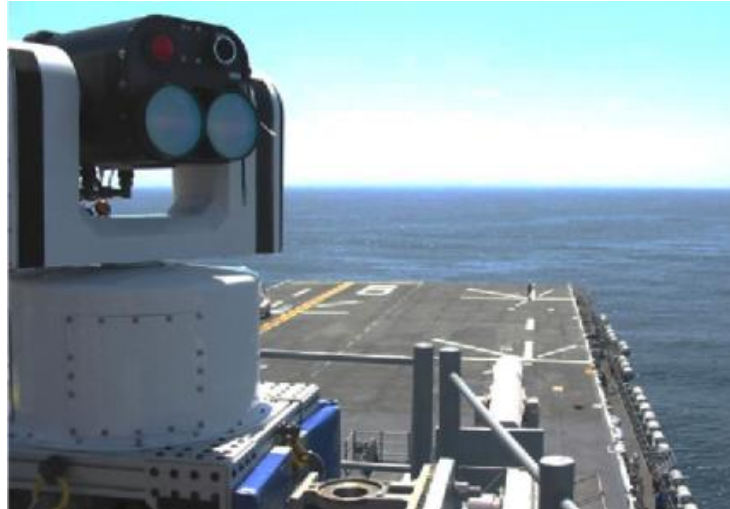
Figure 25. FSO Terminal on USS Bonhomme Richard . Source: [9].
