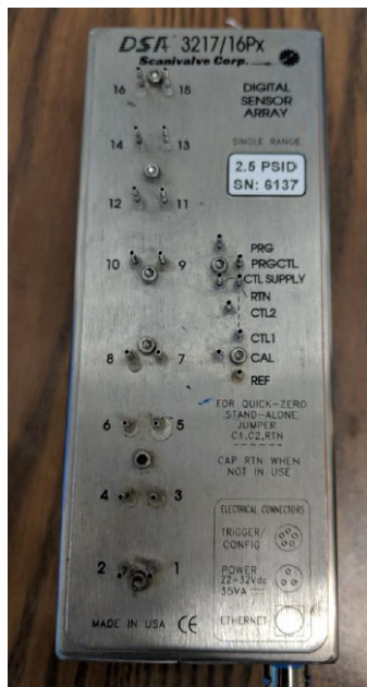
Figure 11. DSA 3217/16Px “Pressure Brick”
