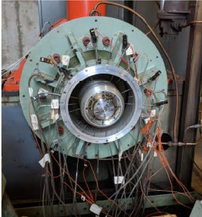
Figure 33. Pressure and Temperature Instrumentation Ports for Outlet Casing
