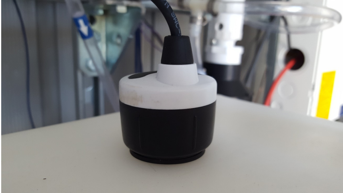
Figure 9. Omega ultrasonic tank level indicator.
