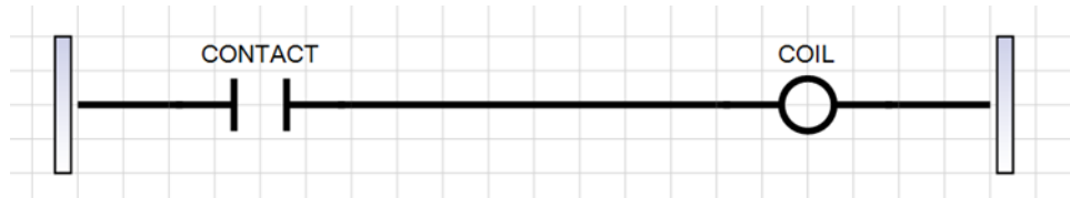
Figure 19. Ladder diagram rung inside function block diagram program.
