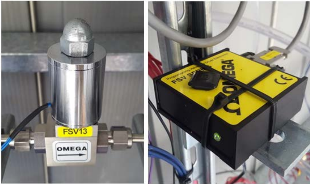
Figure 17. Omega FSV13 proportional control valve and corresponding control box.
